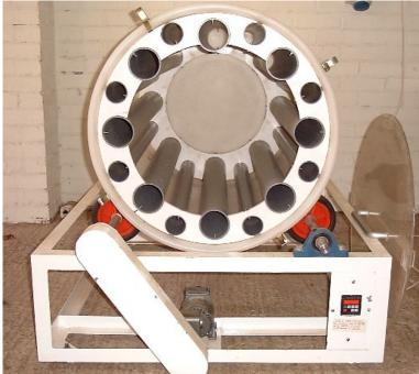
Appendix Figure 4. Motor drive unit and drum used to simulate conditions suffered by onions during commercial handling.
